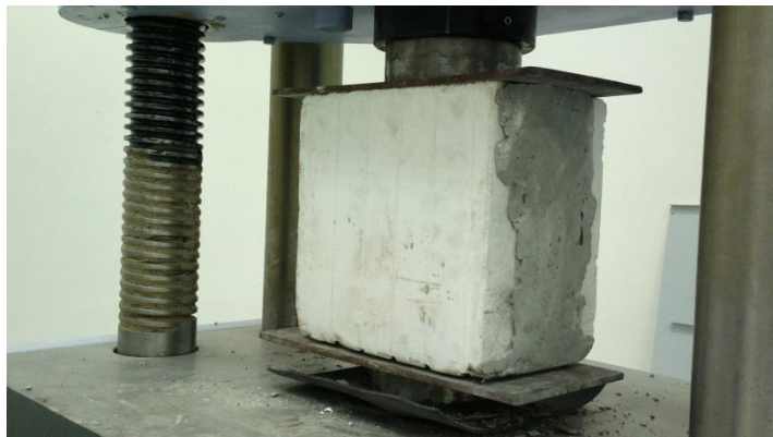
Figure 2. Insulated concrete block under compression test
