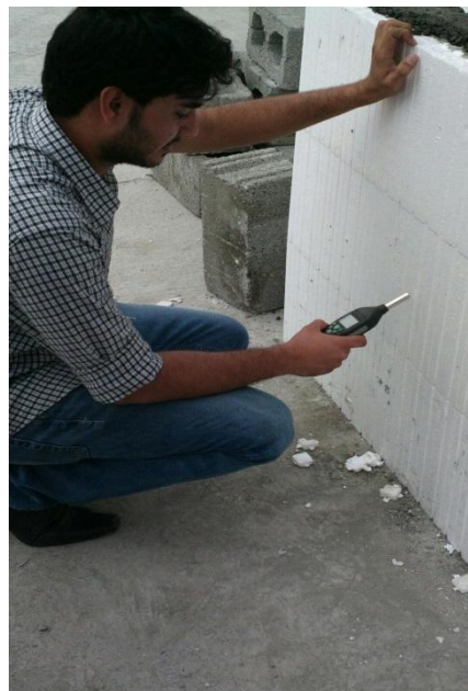
Figure 6. Checking sound passing through room made of Insulated concrete blocks.
