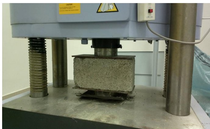
Figure 3. Solid concrete block under compression test
